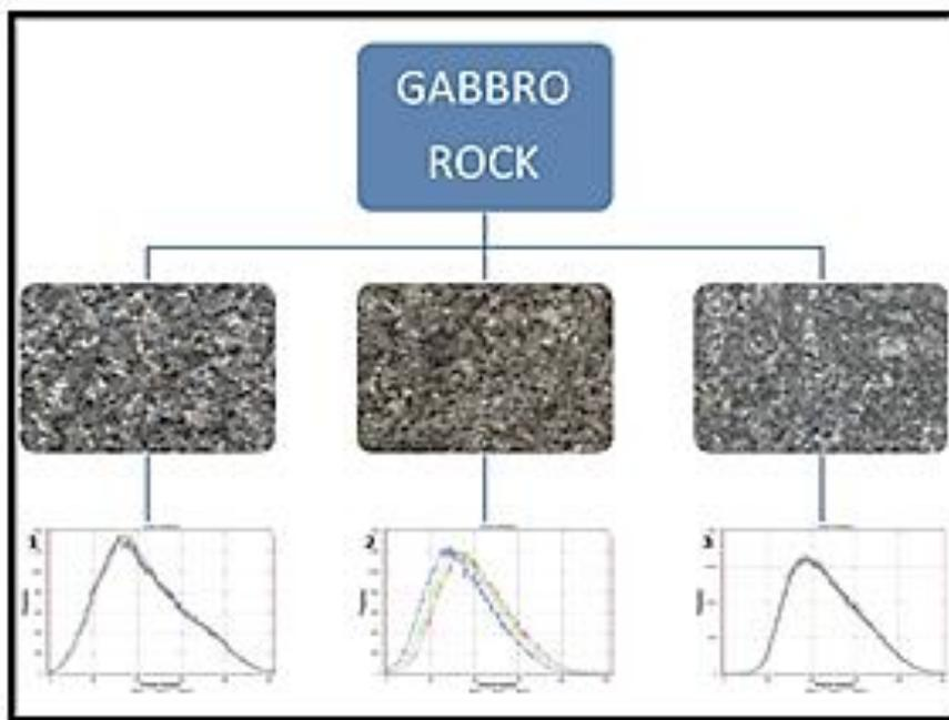
Figure 6 Photograph of various hand specimens of gabbro and their histogram.
